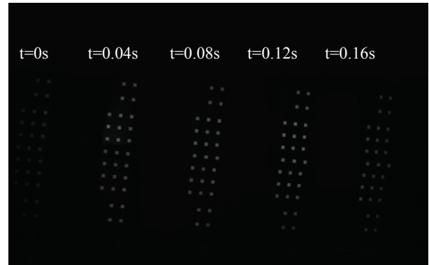
Fig. 7 Sequential images of the glider at every 0.04 sec.
