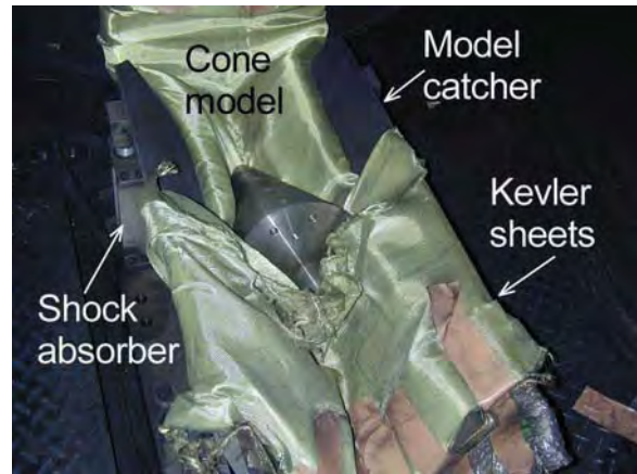
Fig.8 The test model and the model catcher immediately after the wind tunnel shot (#1923). The blunted cone successfully soft landed on the catcher without any damage. Model and data-logger have been reused through the present test campaign.
