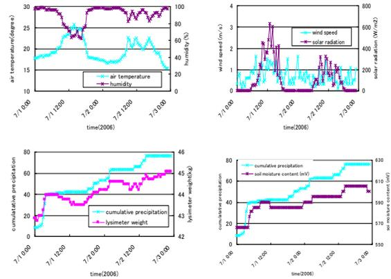
Figure 6. Examples of meteorological data and soil information data on July 1-3 by Field Server system.
