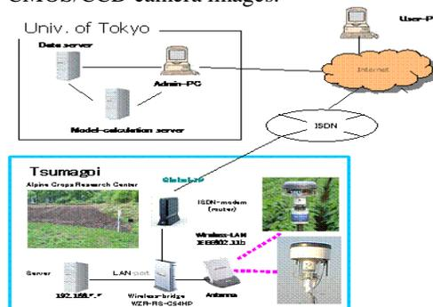
Figure 2. Field Server monitoring system.
