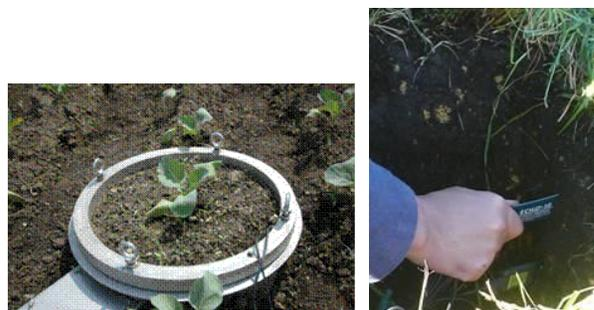
Figure 3. Lysimeter and soil moisture sensor.
