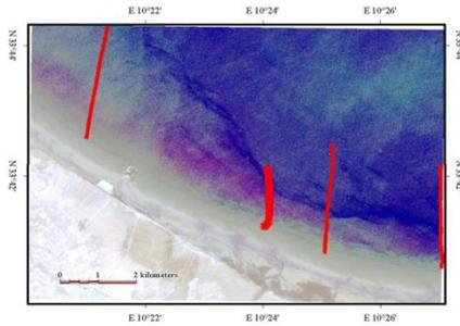
**Fig. 5** Enhanced AVNIR2 imagery of Zarat and sidescan sonar survey lines (red) to obtain ground truth
