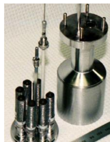
Fig. 1 AMPS-NASA PX-8 cell (21% efficiency, power density 60 \text{ kWe}/\text{m}^3 ) 2)
