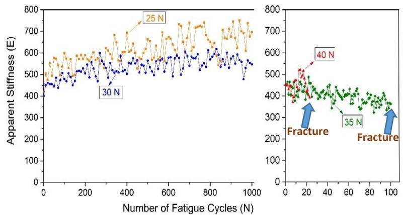
Fig.5 Apparent Stiffness vs Number of Fatigue cycles
