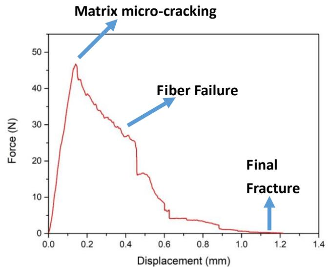
Fig. 3 Force vs cross-head displacement at 1100°C
