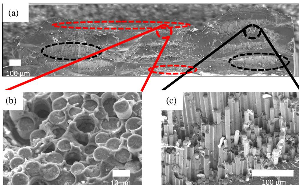
Fig. 6 SEM microstructures after 40 N fatigue test at 1100C showing (a) Fracture surface, (b) Brittle fracture region and (c) Fiber pullout region
