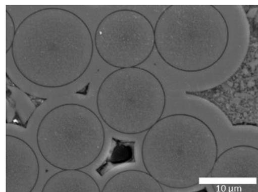
Fig.2 SEM cross sectional image of SiC/SiC CMC
