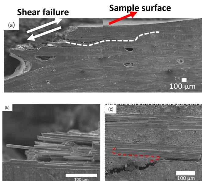
Fig. 4 SEM fracture microstructures after 1100°C compression test showing (a) crack propagation, (b) fiber pullout and (c) crack deflection
