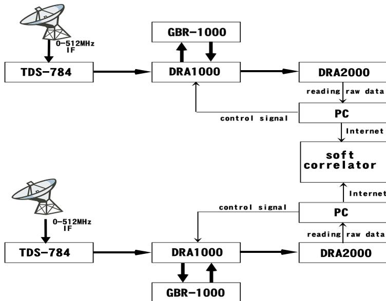
Figure 2: Real time fringe check system diagram
