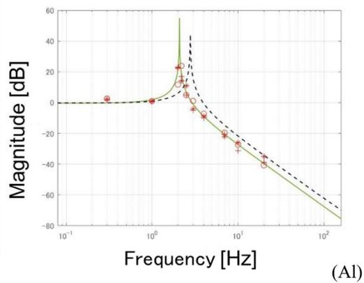
Fig.10 Horizontal vibration transfer characteristics
