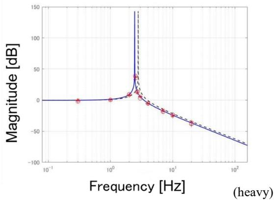
Fig.5 Horizontal vibration transfer characteristics
