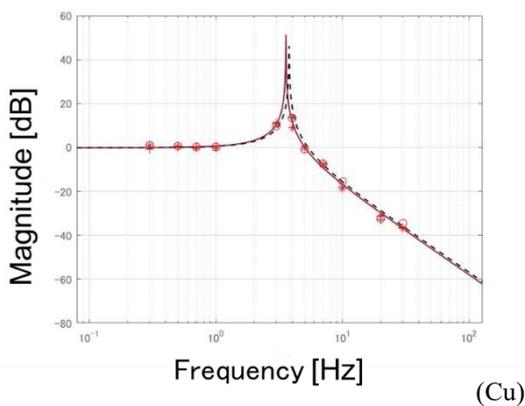
Fig.7 Vertical vibration transfer characteristics
