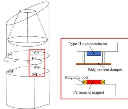
**Fig.2 Micro Vibration Disturbance Suppression Mechanism**
