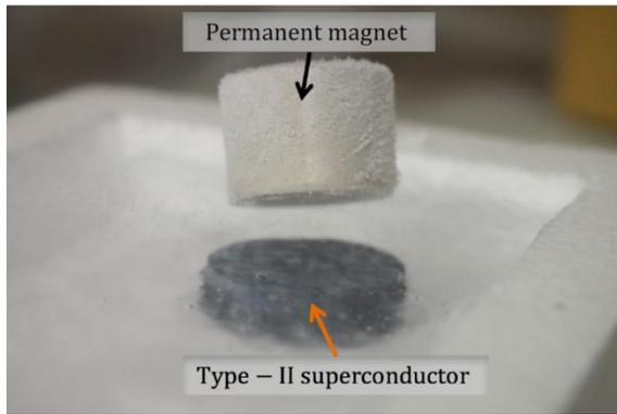
**Fig.1 Magnetic flux pinning effect**
