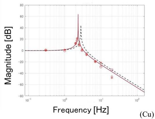
Fig.8 Horizontal vibration transfer characteristics
