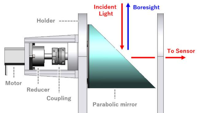
**Figure 1.** 3D CAD images of TCAP tracking mirror without covers
