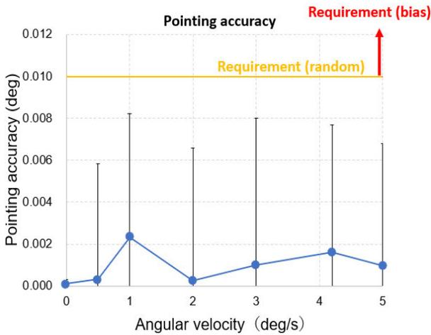
**Figure 3.** Pointing accuracies and stabilities of TCAP actuator BBM.
