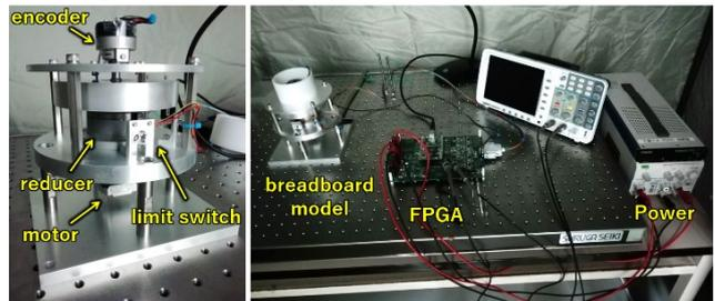
**Figure 2.** Breadboard model (BBM) of TCAP actuator (left) and configuration for evaluation test (right).
