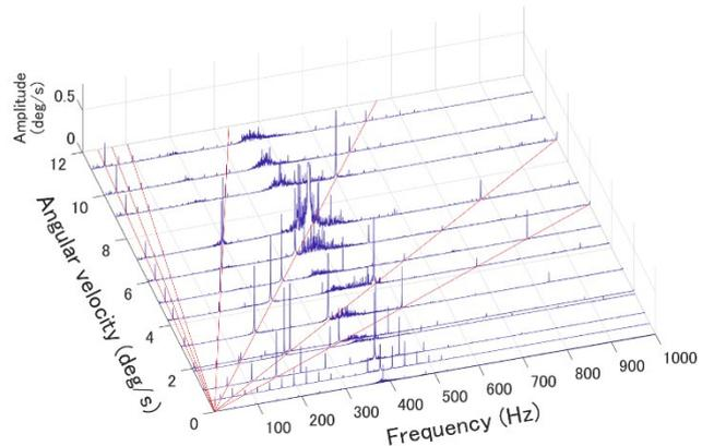
**Figure 4.** Waterfall plot of frequency analyses of the angular velocities measured by the encoder. Red lines show the frequencies related to motor pulses.
