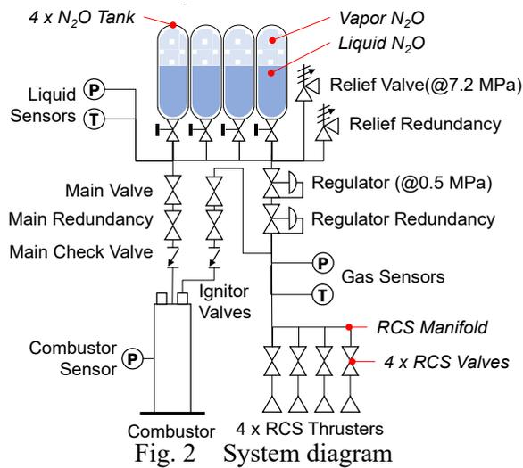
To confirm the thrust performance of the kick motor for the evaluation of success level, as well as for ensuring the safety of the experiment team, a minimum of three pressure measurements and two temperature measurements must be taken with a sampling rate of 10 Hz or more. These measurements are summarized in Table 2 below.
