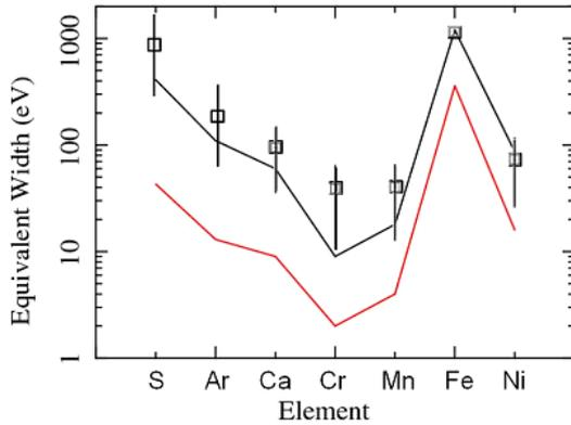
Fig. 3. Equivalent width of  $K\alpha$  line of various neutral atoms. Black and red lines show values in the X-ray and electron scenarios calculated by Geant4, respectively. The data points marked with square are observed value in our work. Errors are estimated at the 90% confidence level.
