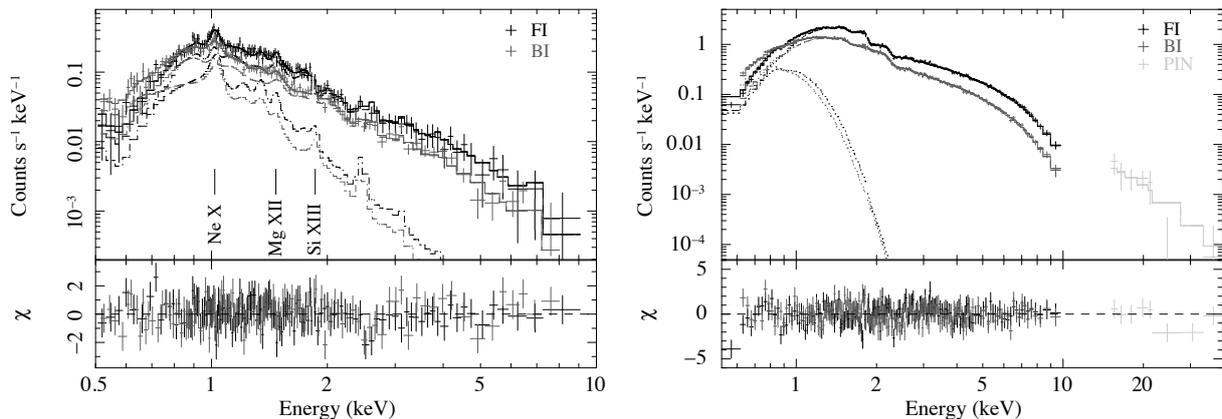
Fig. 1. Spectra of 1RXS J165256.3–264503 (left) and 1RXS J174459.5–172640 (right). The data obtained with FI CCD, BI CCD, and HXD PIN are indicated with black, red, and green crosses. We superposed the best-fit model on the data, together with each component.
