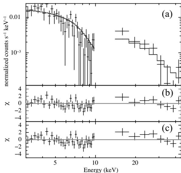
Fig. 2. The second component of MCG-6-30-15 fitted with `compTT` (a and b), or power-law (c)
