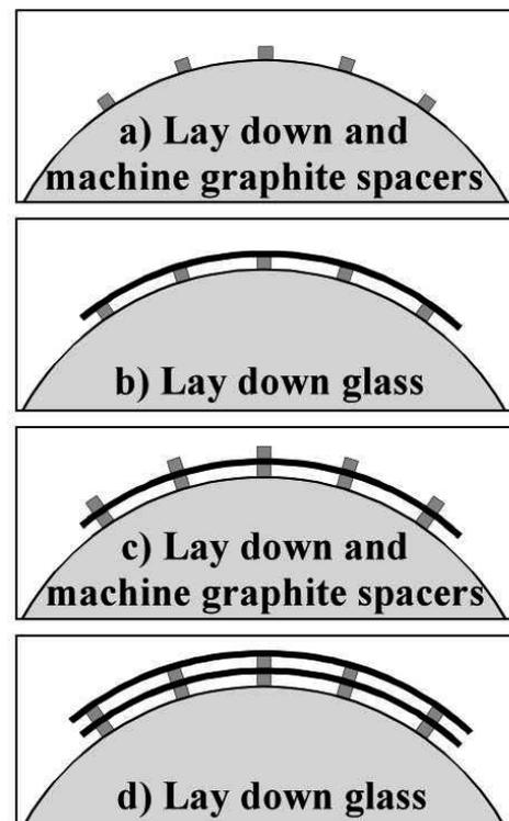
Fig. 4. Fabrication of glass-graphite-epoxy composite optics
