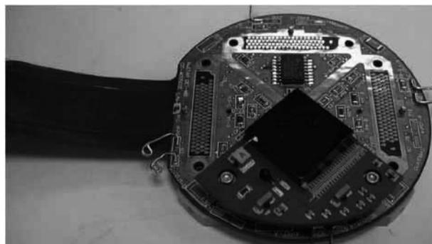
Fig. 6. One of four CdZnTe pixel hybrids on the focal plane motherboard
