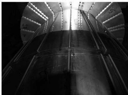
Fig. 5. NuSTAR prototype telescope. The segmented glass and spacers are visible on the Titanium mandrel
