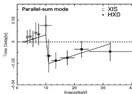
Fig. 3. Relative shift of the time variations between different energy bands taking 2-3 keV as a reference. Possible jump at  $\sim 10$  keV represents the time assignment error of the XIS.
