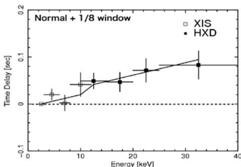
Fig. 2. Relative shift of the time variations between different energy bands of Cyg X-1 data taking 2-3 keV as a reference. Possible jump at  $\sim 11$  keV represents the time assignment error of the XIS.
