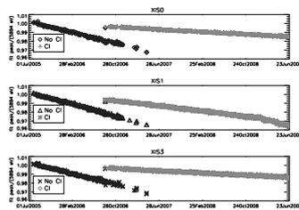
Fig. 3. Energy Scale Trend without Gain Corrections
