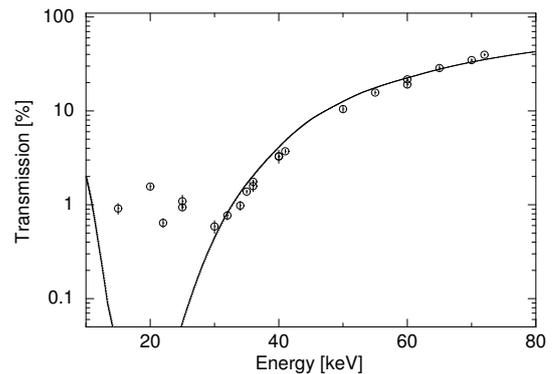
Fig. 2. EUV transmission of the polyimide of OBL as a function of EUV energy. The model line is assumed the thickness of polyimide is  $1100\text{\AA}$ .
