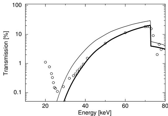
Fig. 1. EUV transmission of the OBF as a function of EUV energy. The Al-L edge absorption structure above  $\sim 70$  eV is clearly seen.
