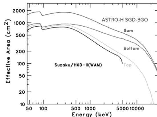
Fig. 1. Comparison of effective area between SGD-BGO and HXD-WAM.
