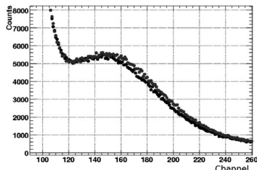
Fig. 2.  $^{241}\text{Am}$  (59.5 keV) spectrum with a large BGO plus a small APD. Colors of data indicate the difference among the readout positions of APD to BGO.
