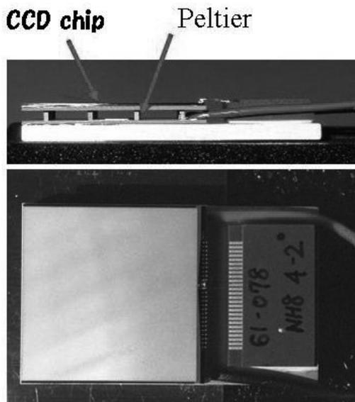
Fig. 2. X-ray CCD of MAXI
