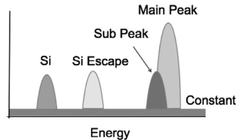
Fig. 3. Responses function of CCD, consists of 4 gaussian components and a constant component.
