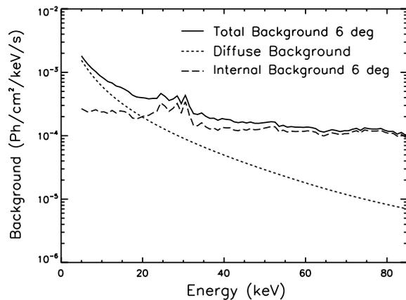
Fig. 1. Simulated background at 6 degree equatorial orbit
