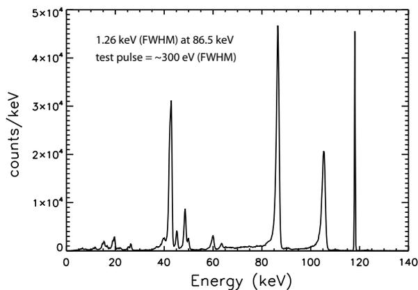
Fig. 2. Eu-155 source spectrum observed with NuSTAR prototype detector at 0°C
