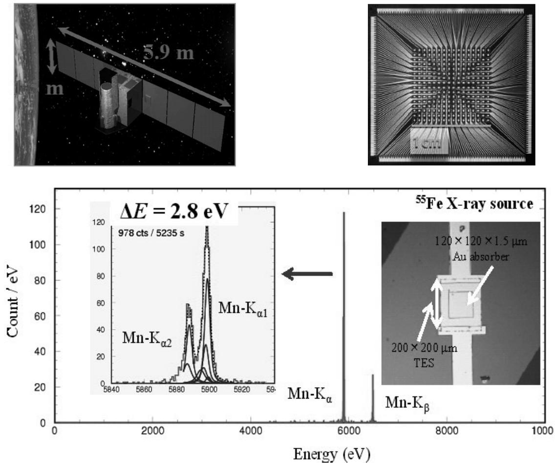
Fig. 1. Upper left: The DIOS spacecraft. Upper right: A picture of the 16 $\times$ 16 TES array. Lower left: Energy spectrum for  $^{55}\text{Fe}$  X-ray source by a single pixel TES calorimeter. Lower right: the fabricated Ti/Au TES calorimeter with Au absorber.
