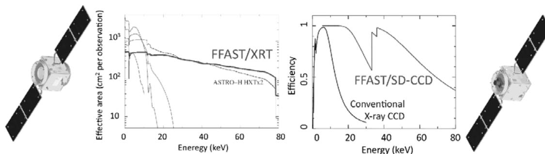
Fig. 1. *FFAST* configuration in orbit. (left : the telescope satellite, right : the detector satellite). The effective area of the *FFAST*/XRT (middle left). The detection efficiency of the SD-CCD (middle right).
