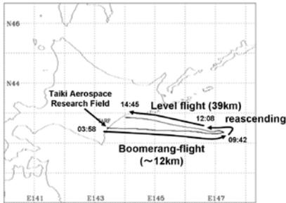
Fig. 2. Flight route of balloon. We obtained a level flight for 2.5 hours at an altitude of about 39km.
