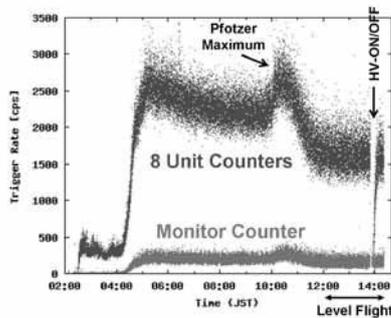
Fig. 3. Trigger rates of the 8 unit counters and the monitor counter. These rates change drastically at the time which corresponds to launching and reascending.
