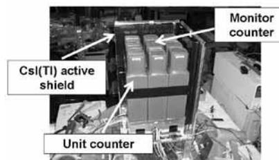
Fig. 1. Flight model of PHENEX polarimeter. Eight unit counters and one monitor counter are installed in CsI(Tl) active shields.
