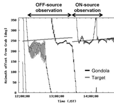
Fig. 4. Azimuthal angle of the gondola during level flight is drawn. Unfortunately, the duration which the Crab remains at the field of view of the PHENEX polarimeter was about 10 minutes because the ACS did not function correctly
