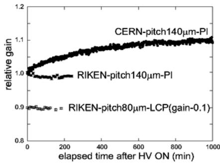
Fig. 1. Short-term gain stability of the RIKEN and CERN GEMs. The time-zero means the moment of turning on high voltage. The gain is normalized at the time-zero.
