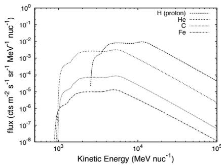
Fig. 2. The flux of incident particles assuming an orbit at an altitude of 600 km and inclination of 30 degrees. The flux is calculated by CREME96: FLUX DRIVER.
