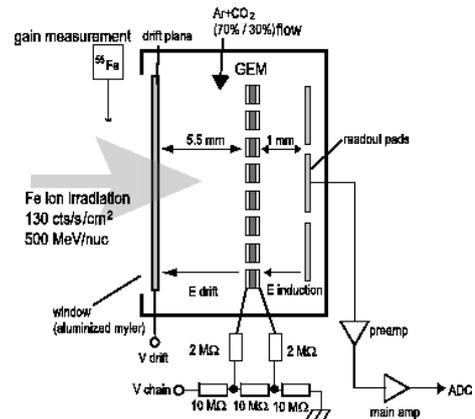
Fig. 3. Setup of irradiation test. Full-striped Fe ion beam comes from the synchrotron accelerator, HIMAC.
