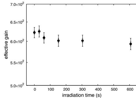
Fig. 4. Gain variation during the Fe ion irradiation test. The gain was obtained by using a <sup>55</sup>Fe source. The error bars show statistic and systematic errors. The data point at 607 s corresponds to the 40-year equivalent cosmic-rays.
