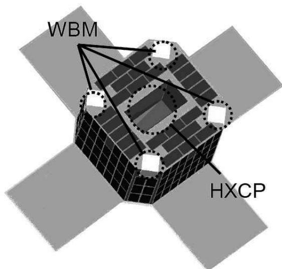
Fig. 1. Tsubame configuration: Hard X-ray Compton Polarimeter (HXCP) is centered at the observatory. CsI counters of the Wide-field Burst Monitor (WBM) are attached to each corner of the observatory.
