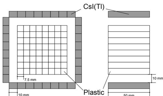
Fig. 2. Detector design for hard X-ray Compton polarimeter (HXCP): CsI scintillators (absorber) surround plastic scintillators (scatterer).
