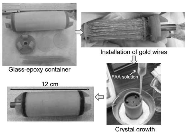
Fig. 1. Fabrication of FAA salt pill.
