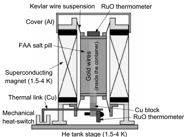
Fig. 2. Setup of the salt pill
