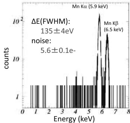
Fig. 3. A <sup>55</sup>Fe spectrum taken by an EM ASIC and a baseline CCD chip.
