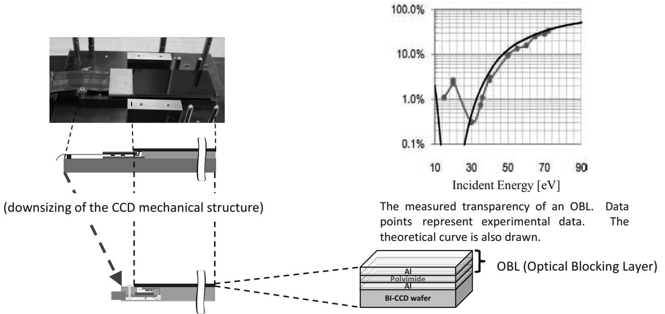
Fig. 1. Baseline (upper-left) and current (lower-left) designs of FPA quadrants and the optical blocking layer design (right).
