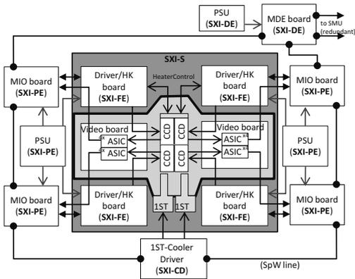
Fig. 2. A schematic drawing of the SXI components and the electrical connections between them.
