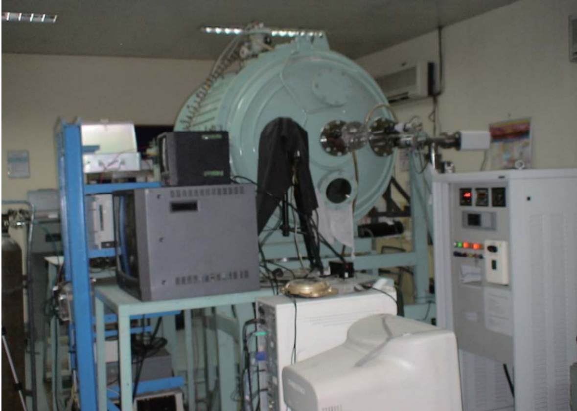
HV Power supply and Pumping unit
