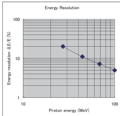
Fig. 5. The energy resolution of the sensor
