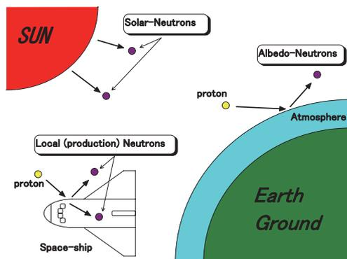
the neutron instrument at SEDA. The neutron measurement module will extend to about 1 meter in order to avoid the neutrons which are produced by the collisions between the wall of SEDA, the main body and protons as shown in Figure 2.
