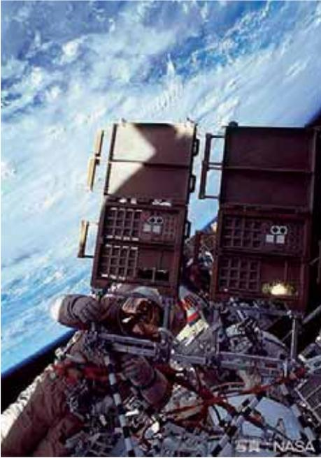
**Fig. 8** EVA for deconstructing SM/MPAC&SEED #1 (August 2002)
