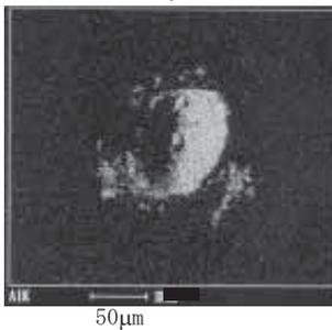
(b) EDX mapping image. Light dots show Al components of the same area of the SEM image.
