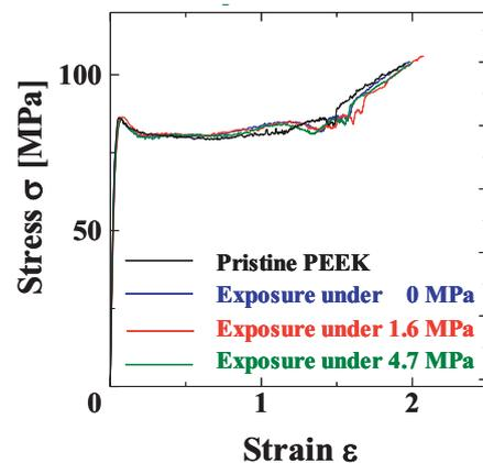
Fig.14 Stress-strain curves of the AO irradiated samples with a fluence of  $2.79 \times 10^{20}$  atoms/cm<sup>2</sup>.
