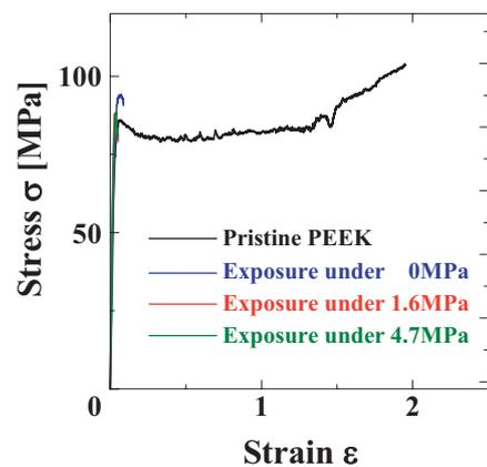
Fig.15 Stress-strain curves of the UV irradiated samples with a fluence of 34ESD ( $3.47 \times 10^4$  J/cm<sup>2</sup>).
