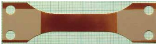
Fig.12 Surface appearance of the UV irradiated sample (34ESD ( $3.47 \times 10^4$  J/cm<sup>2</sup>), under 4.7MPa).
