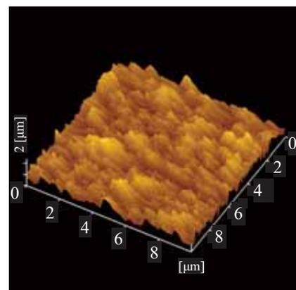
Fig.11 Surface morphology of the AO irradiated sample ( $2.79 \times 10^{20}$  atoms/cm<sup>2</sup>).
