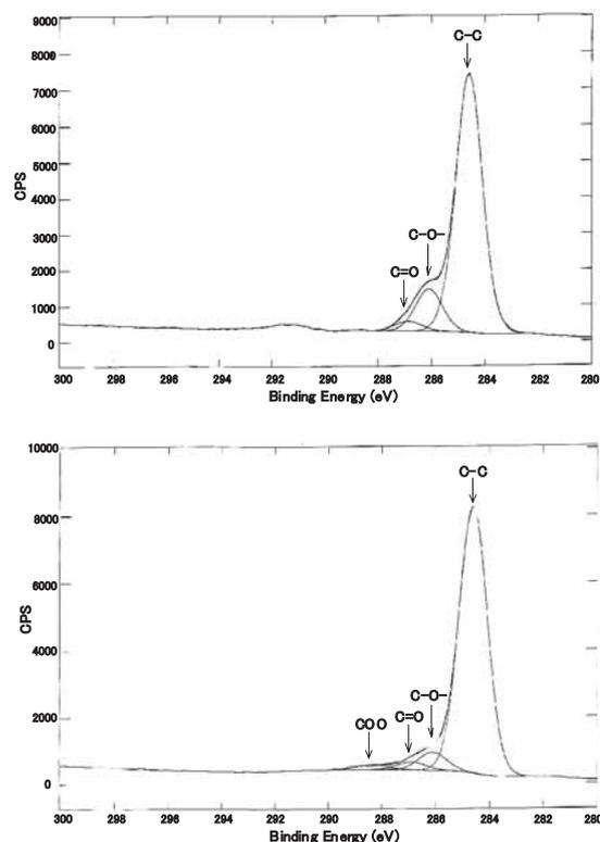
**Fig.17** XPS analyses before and after UV irradiation.
