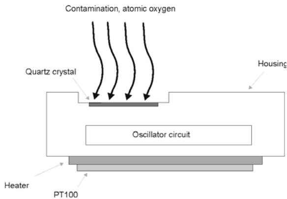
Figure 3 : QCM sensor in operational mode
