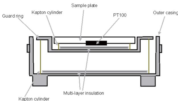
Figure 6 Micro-calorimeter schematic
