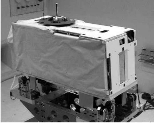
Fig. 3. The Monitor of All-sky X-ray Image (MAXI) flight model, which will be attached to the International Space Station in 2009.
