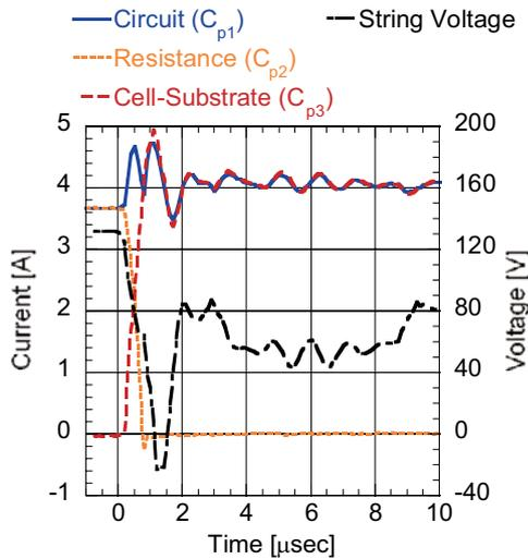
Fig. 6 Current and voltage of onset of arcing
