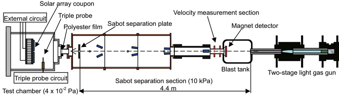
Fig. 1 Experimental setup of hypervelocity impact test
