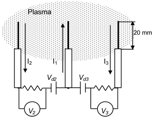
Fig. 4 Triple probe circuit
