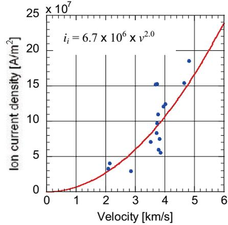
Fig. 7 Ion current density at impact point
