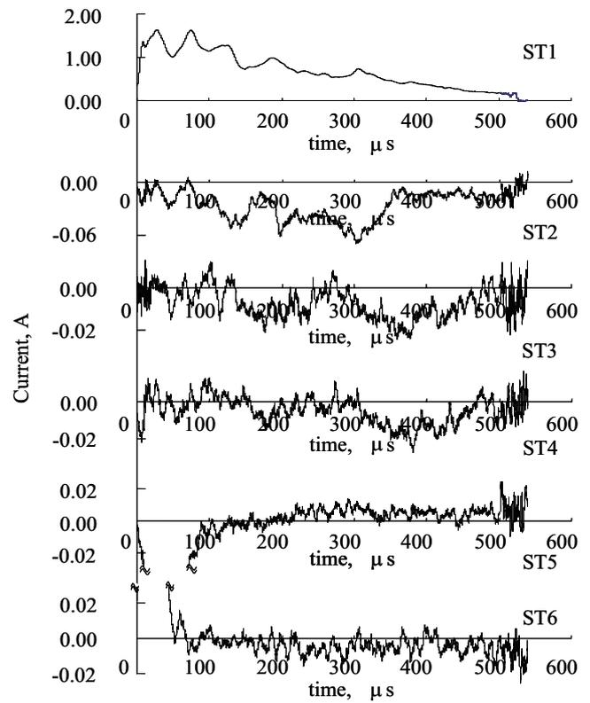
Fig. 6. The typical current waveforms for the arc that occurred at ST1.
