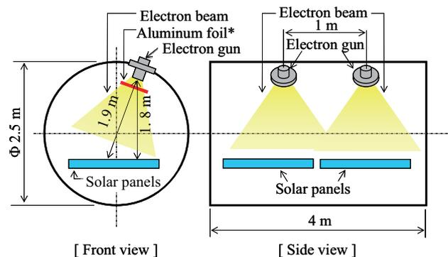
\* Al foil was used to expand the irradiation area of electron beam.
