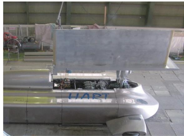
Fig. 4 Vertically installed flat plate on HART vehicle
