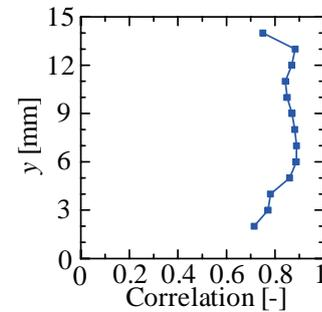
Fig. 6 Correlation coefficients between each hot-wire output.
