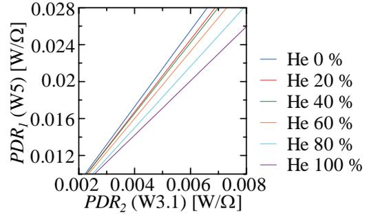
Fig. 10 Calibration map used for detecting helium concentration.
