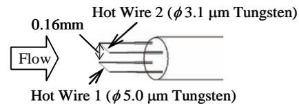
Fig. 1 Double-hot-wire probe.
