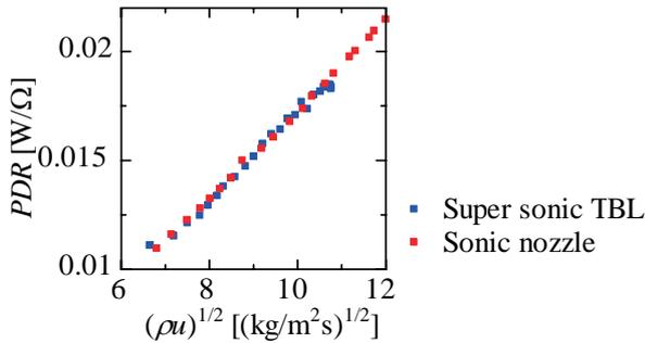
Fig. 3 Calibration results in sonic flow and in Mach 2.4 supersonic turbulent boundary layer.
