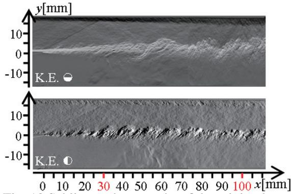
Fig. 13 Schlieren photographs of the mixing layer.
