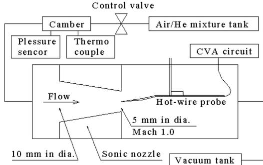
Fig. 2 Sonic nozzle calibration apparatus.
