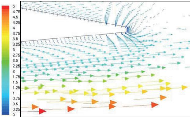
Fig.7 Velocity vector around the trailing edge ( $U=5[m/s], \phi=5\pi/6, h/b=0.75, Re=3.4 \times 10^4$ )
