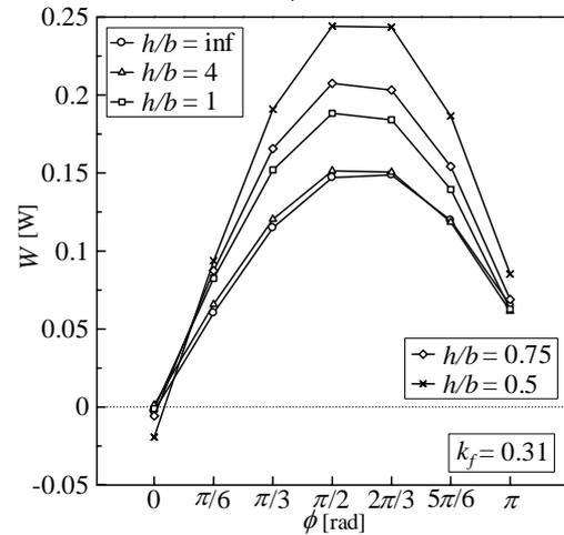
Fig.9 The dependence of aerodynamic work on phase for  $U = 15m/s$  (upper) and  $10m/s$  (lower) lag between the heaving oscillation and the pitching oscillation. It is well known that the maximum work id done near  $\phi = \pi/2$ , fig.9 shows that the ground increases the work.
