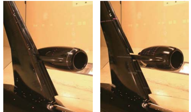
Fig.8 Two types of the nacelles. Left: Long-cowling, right: Short-cowling
