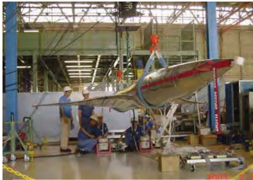
Fig.3 NEXST1 under vibration test
