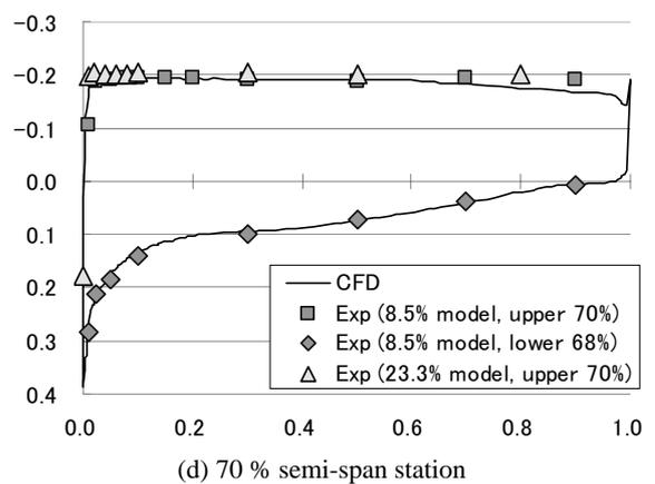
Fig. 5  $C_p$  distributions at  $2^\circ$  angle of attack
