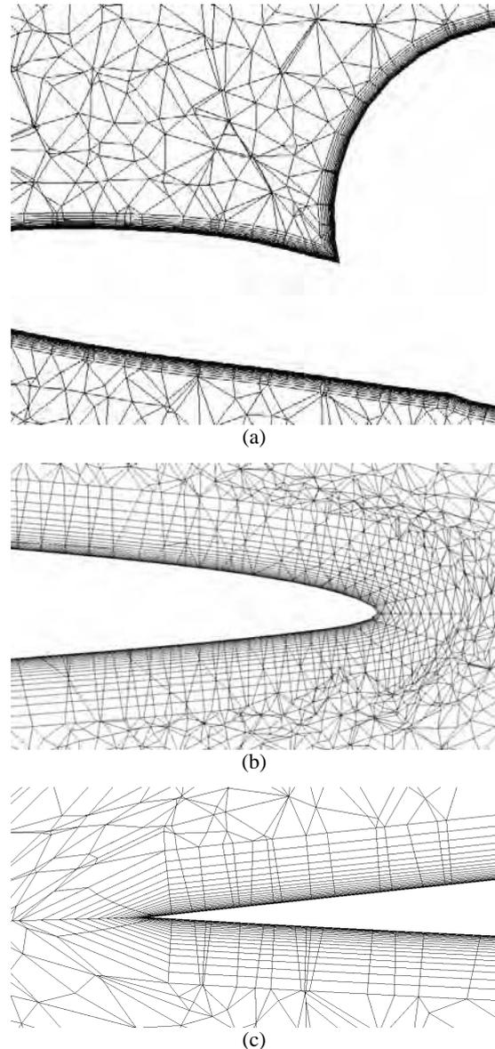
Fig. 2 Hybrid mesh: (a) cross-flow cross section at  $x = 0.5$ ; (b) spanwise cross section near the wing leading edge at 30% semi-span station; (c) the same section near the tailing edge
