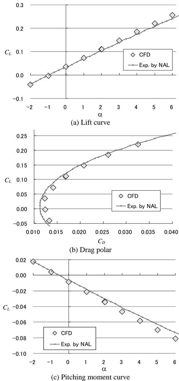
Fig. 3 Lift curve, drag polar and pitching moment curve for NAL experimental airplane ( $M_\infty = 2.0$ ,  $Re = 27.5 \times 10^6$ )
