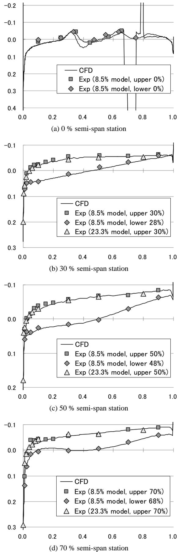
Fig. 4  $C_p$  distributions at 0° angle of attack
