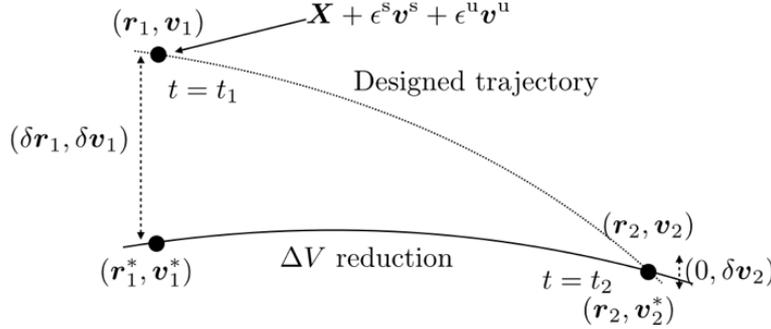
Fig. 8 Conceptual figure of  $\Delta V$  reduction
