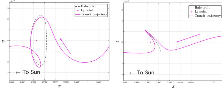
Fig.4 Transit trajectory (left one is looked by x-y plane, right one is by x-z plane)
