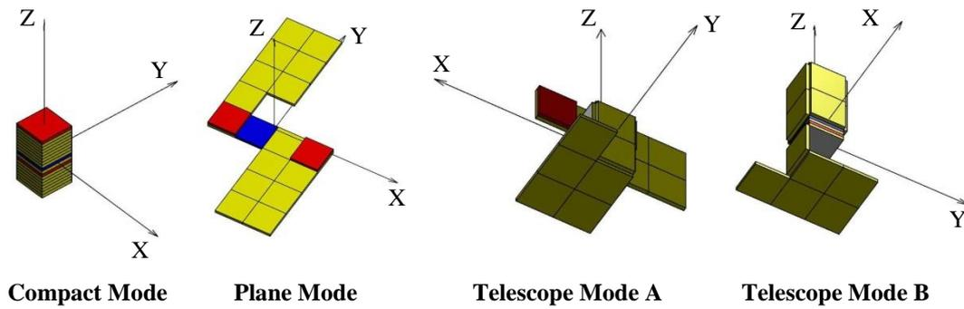
Figure 1. Shape change of a transformable spacecraft
