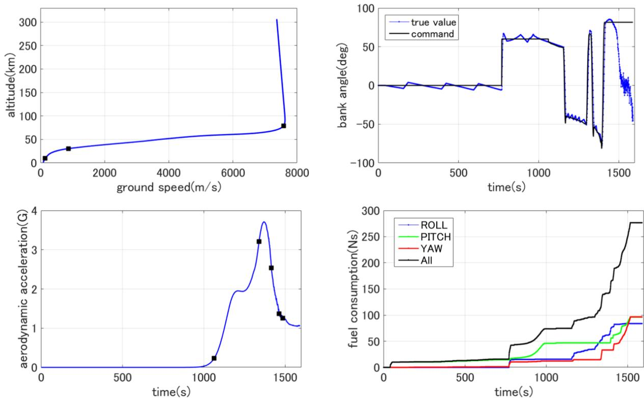
Figure 2.2 Reference trajectory of the HSRC
