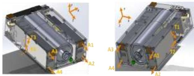
Fig. 3 Thrusters of MiPS
