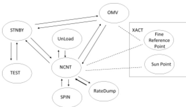
Fig. 5 State transition diagram of AOCS
