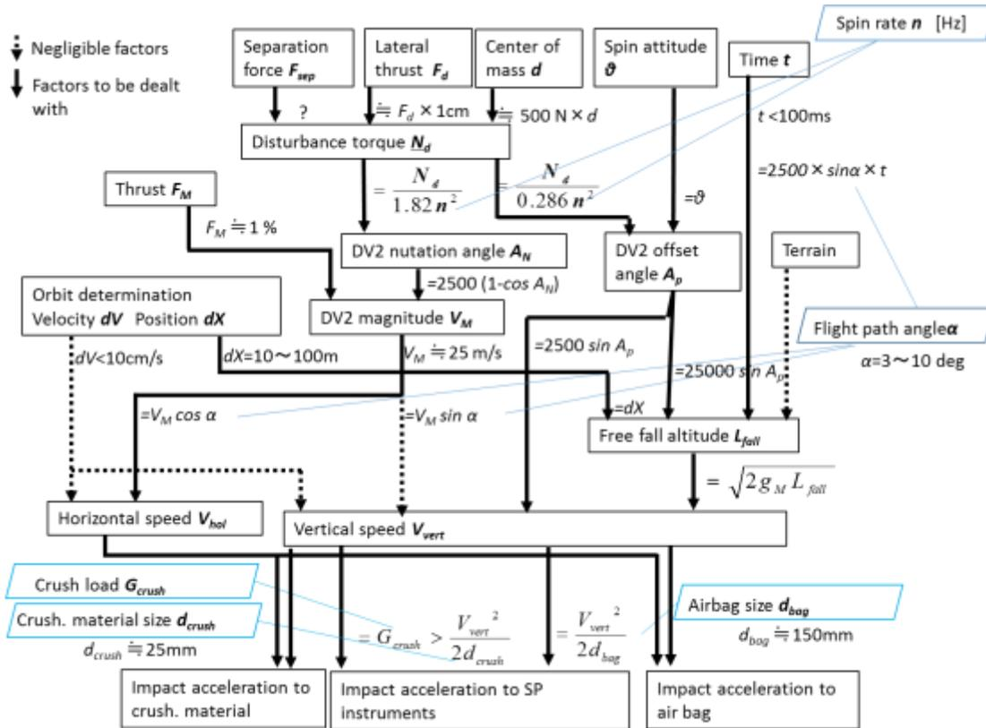
Fig. 6 The error analysis for the impact velocity and acceleration
