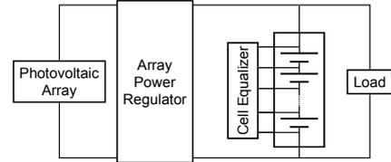
(a) Traditional unregulated power system using series-connected cells.
