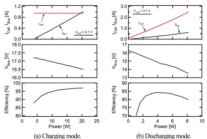
Fig. 5. Measured power conversion efficiencies and bus voltage characteristics.
