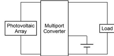
(b) Proposed unregulated power system using a single-cell.
