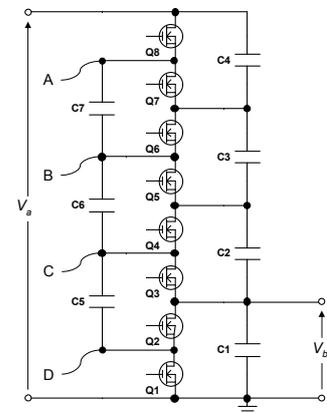
(b) Switched capacitor converter.
