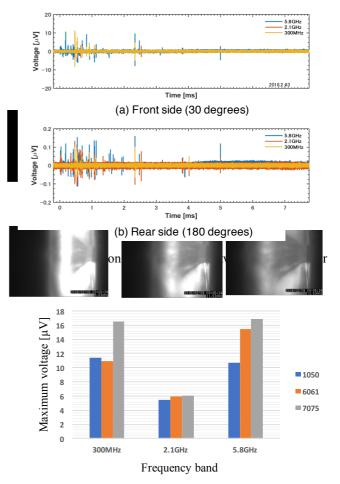
Fig. 7. Comparison of maximum amplitude of microwaves depending on target materials.
