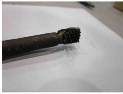
Fig. 3. A photograph of the 16-ch Langmuir probe array, which is set in the pressurized chamber.
